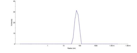
The mean peak Radius of VLP is 50-80 nm with more than 95% intensity as determined by dynamic light scattering (DLS).
