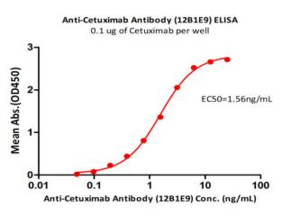
Immobilized Cetuximab at 1  $\mu$ g/mL (100  $\mu$ L/well) can bind Anti-Cetuximab Antibody (12B1E9) (Cat. No. CEB-Y29c) with a linear range of 0.2-1.6 ng/mL (QC tested).
