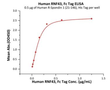
Immobilized Human R-Spondin 1 (21-146), His Tag, premium grade (Cat. No. RS6-H4220) at 5  $\mu$ g/mL (100  $\mu$ L/well) can bind Human RNF43, Fc Tag (Cat. No. RN3-H5256) with a linear range of 0.01-0.156  $\mu$ g/mL (Routinely tested).
