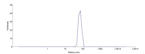
The mean peak Radius of VLP is 60-80 nm with more than 95% intensity as determined by dynamic light scattering (DLS).
